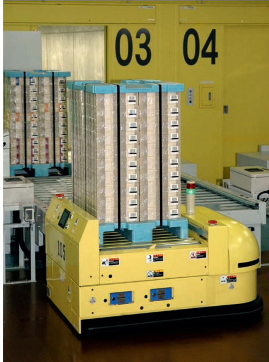
Automatic guided vehicle / Bank of Japan
